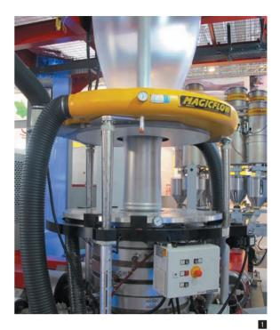
The net effect is that bubble stability is increased, transverse tolerances improved and higher machine outputs are achieved.
